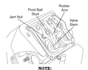
Start all four screws before tightening or it will not be possible to get all the screws in place. Make sure the valve cover gasket is in place.
